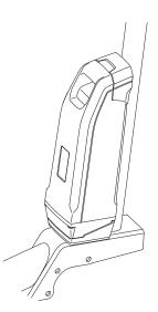
11. Make sure that it is securely attached by pulling the Battery Pack after installation.
